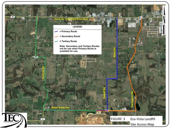
2. Arbor Acres Ave. will be improved from the Eco Vista entrance to the intersection at Dowell Road, on both sides of the street to Collector Street Standards and provide a 12-foot trail along one side of the street. It is currently shown on the north side, but the city may request this be placed on the south side instead.
