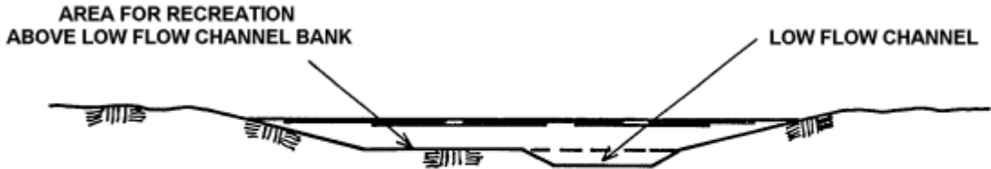
CROSS SECTION WITH LOW FLOW CHANNEL WITH OVERFLOW AREA FOR MAJOR DRAINAGE RUNOFF
