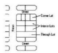
**LOT WIDTHS.** The mean horizontal distance between the side lot lines of a lot measured at right angles to the depth; measurements shall be made at the front building setback.
