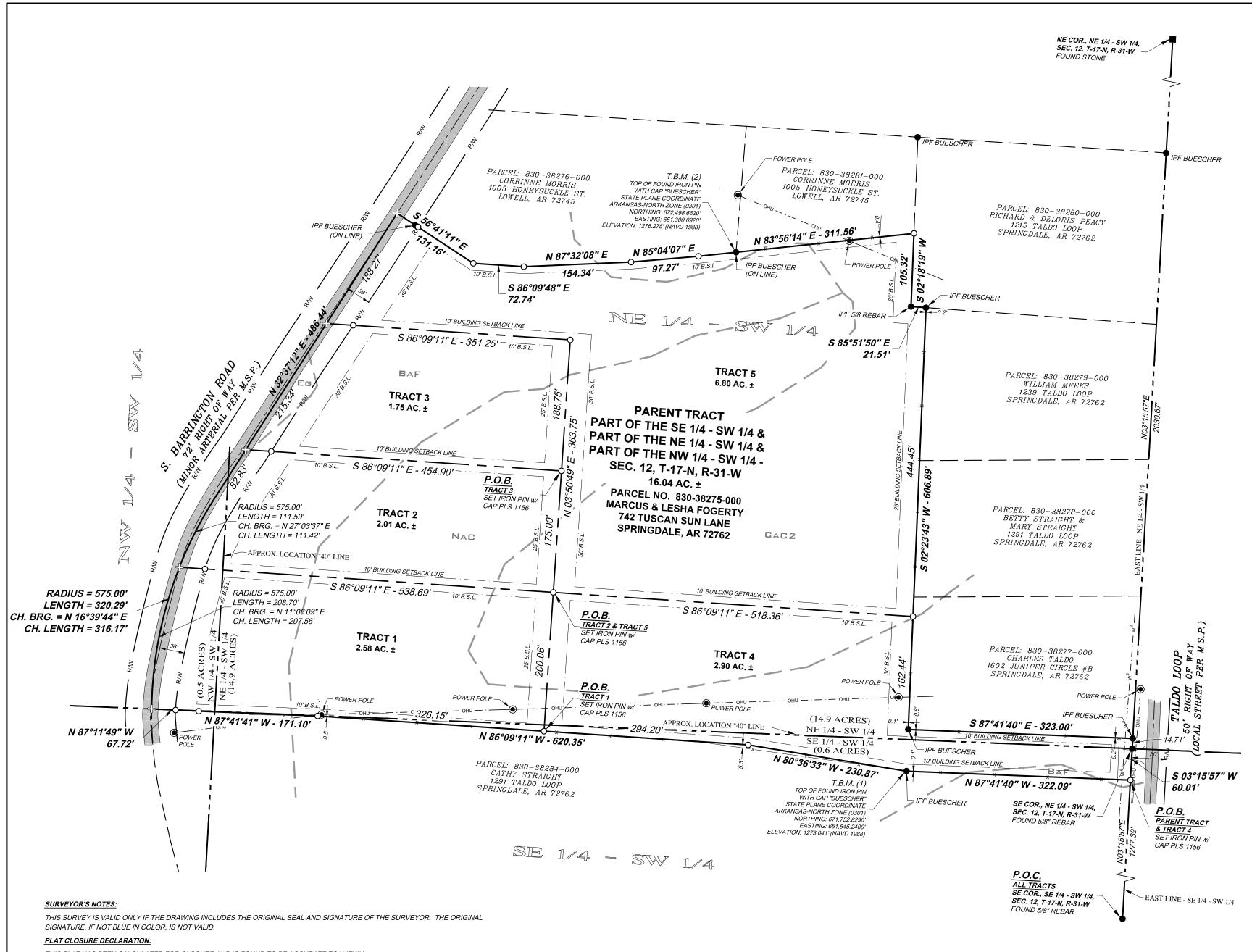
THIS PLAT HAS BEEN CALCULATED FOR CLOSURE AND IS FOUND TO BE ACCURATE TO WITHIN: PARENT TRACT A: ONE FOOT IN 691,860 FEET.
