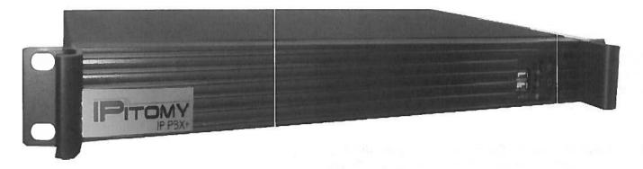
The IPitomy IP1200 is a powerful business communications platform. It is a pure IP PBX designed with exceptional unified communications performance for businesses up to 100 users. The system is compatible with analog lines and T1 /PRI lines for traditional Public Switched Telephone Network (PSTN) connectivity. In addition to traditional telephone lines, the IPitomy IP1200 can use VoIP service providers, replacing traditional PSTN lines with a broadband connection.
