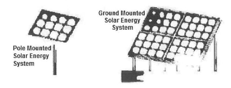
**SOLAR ENERGY SYSTEM, POLE MOUNTED.** A solar energy system with solar panels attached to the top or side of a vertical pole.
