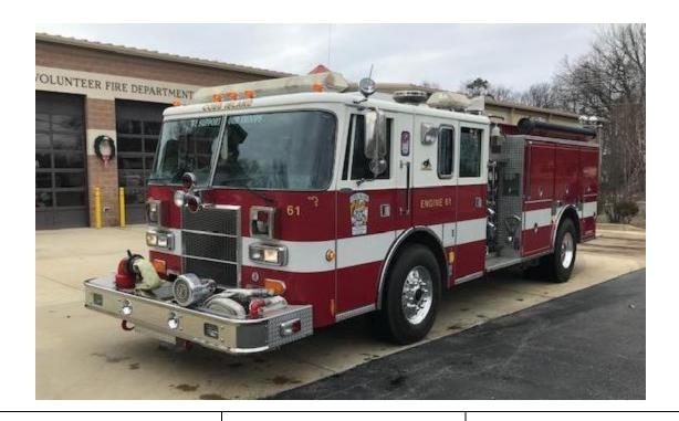
1993 Pierce Pumper Pierce Lance Chassis Seating for 6; 5 SCBA seats 6V92TA 400 HP Diesel Engine Transmission Model: HT740
